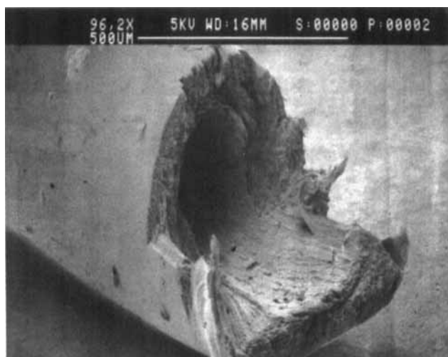
Figure 3. SEM photograph of a fractured melt spun, as-spun fibre of 1b .
